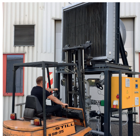
Two-part skid designed for forklift transport
